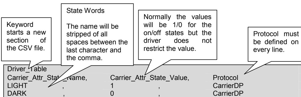
This method may be used to change the values of any of the driver's default state words by duplicating the word and specifying a new value in the configuration file.
